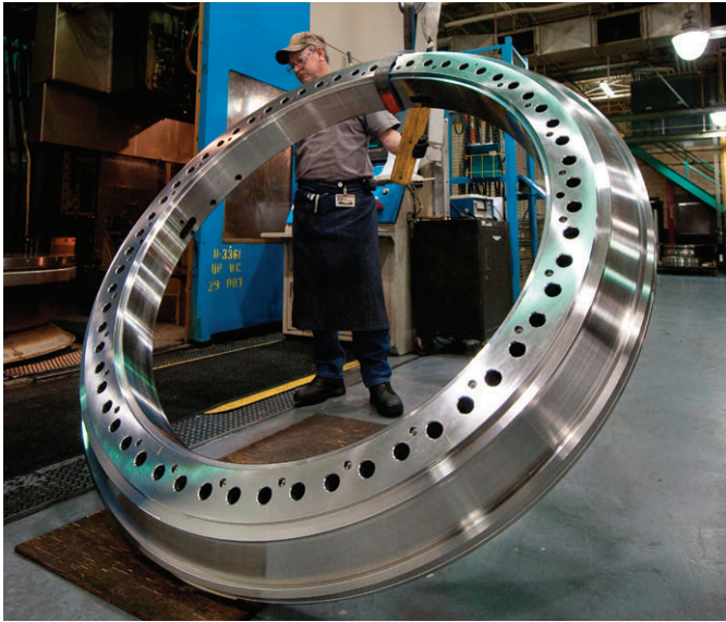
A technician at Timken's Tyger River, South Carolina facility hoists a main-shaft bearing produced at the facility. (Courtesy of The Timken Co.)
